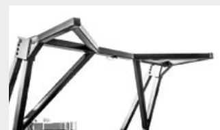
Mechanical push frame guides and pushes material away from carrier
