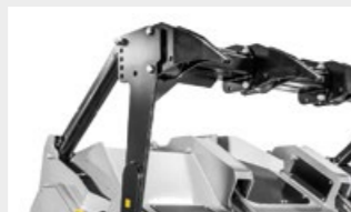
Mechanical/hydraulic push frame guides and pushes material away from carrier
