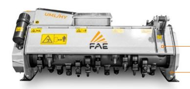
Steel counter-blades helps mulch material into a smaller final size
